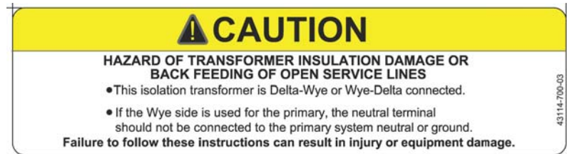
Figure 32: Caution Label for Delta Wye or Wye Delta Connected Transformers
