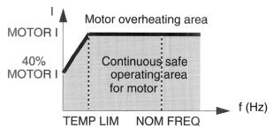
The operation curve can be customized to protect motors with any constant torque speed range.
