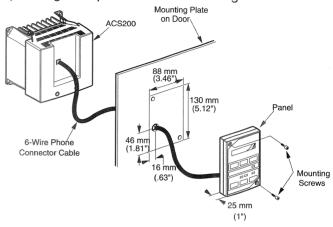
The Keypad Panel also acts as a parameter copy unit that allows the parameters to be copied from one drive to another.
