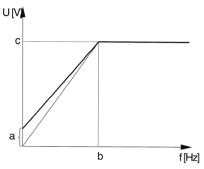
This provides for higher voltage at low speeds anytime during operation (not just at initial start-up; i.e. start function with torque boost). In Automatic, the IR Compensation voltage is set automatically as a function of effective motor current. In Manual, both the IR-Comp Voltage and IR-Comp Range are adjustable.
