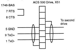
In the modbus communication manual for the ACS 500 there are detailed description for wiring, grounding, and for proper termination of communication cable.
