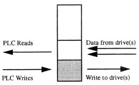
The data is transferred independently from the communication module to the drives, and from the communication module to the PLC. The addresses on the communication module buffer do not match the actual drive addressees.
