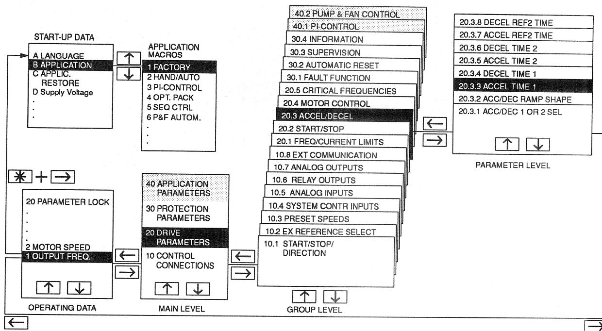
Figure 2-5 shows how to set Parameter 20.1.1 (Minimum Frequency) to 3 Hz starting from Operating Data Parameter 1 (Output Frequency).
