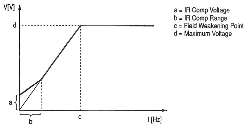
Changing the motor base frequency automatically changes this value if it is set higher than the motor base frequency.
