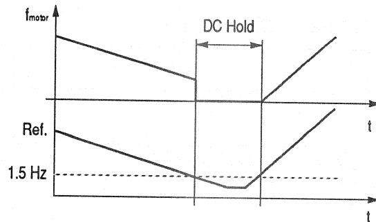
When both reference and output frequencies drop below 1.5 Hz, the drive will stop generating sinusoidal current and inject DC into the motor. The voltage value is the voltage set in the DC Hold Voltage. When the reference frequency goes above 1.5 Hz, the DC will be removed and normal drive function resumes.
