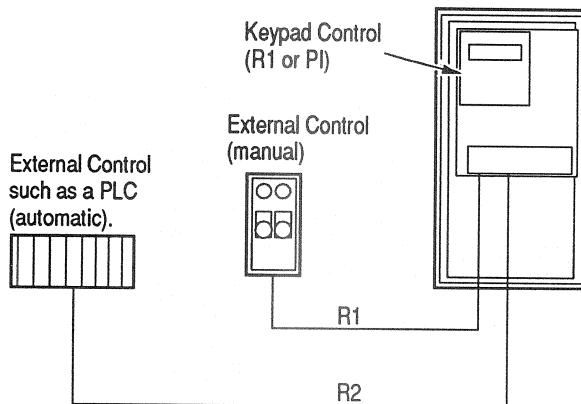
Select Operating Data Parameter 9 (Control Location), then select KEYPAD R1 for keypad control or EXTERNAL for external control. The valid control location is indicated on the display. Square brackets around the Direction and Run indicators on the LCD Display mean Keypad control. No square brackets means External control. R1 on the LCD means Ref 1 and R2 means Ref 2.
