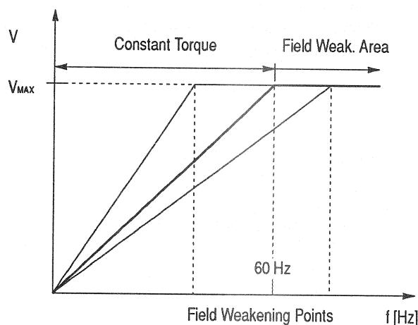
Figure 6-8 shows Parameters 20.4.2 and 20.4.4 adjusted to run a motor not of rated voltage.
