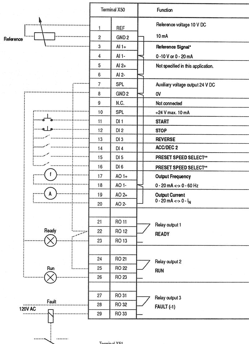
\* Select voltage or current reference with plugs S1 and S2 on the customer interface board (beside the screw terminals 1-6 of X50).
