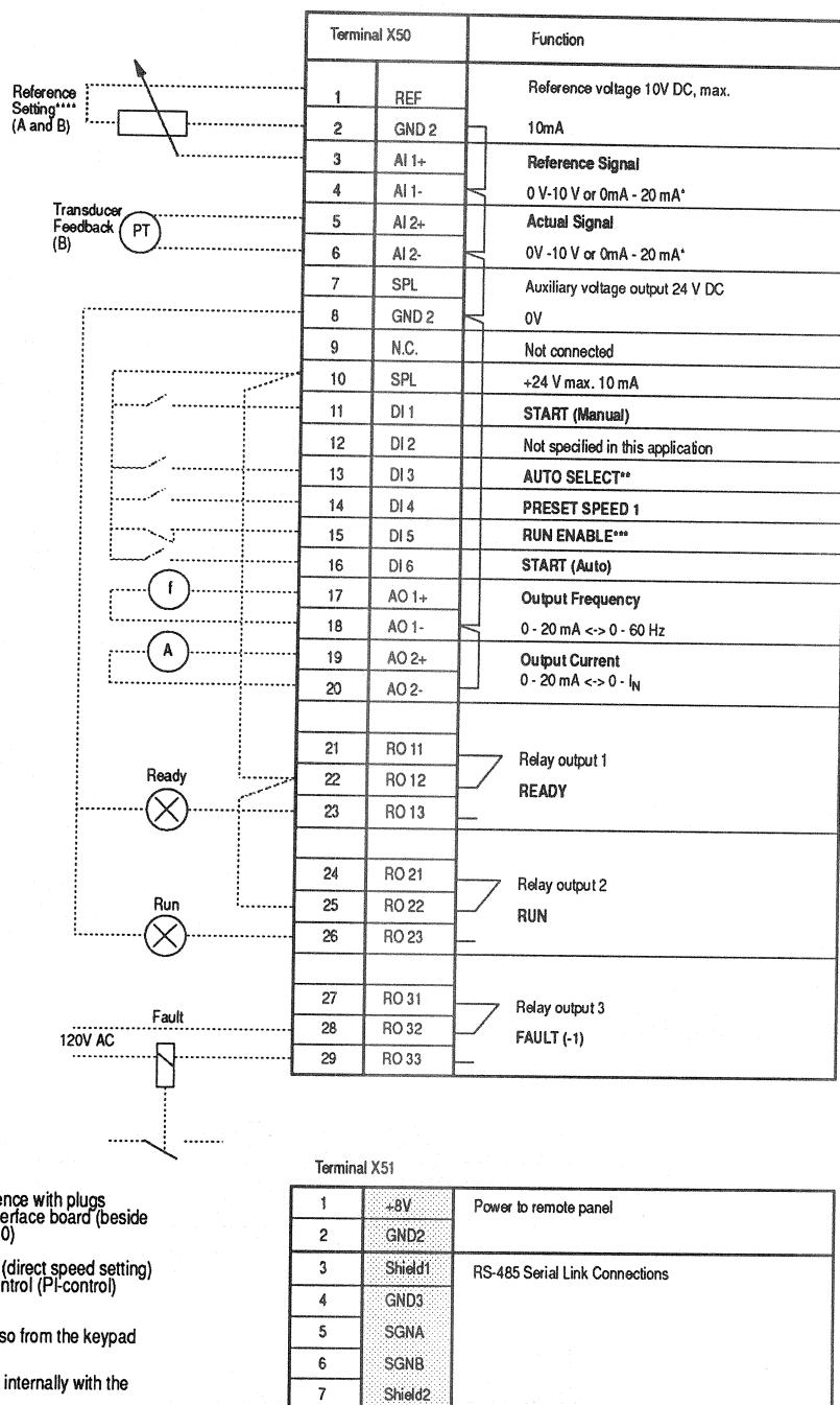
\* Select voltage or current reference with plugs S1 and S2 on the customer interface board (beside the screw terminals 1 - 6 of X50)
