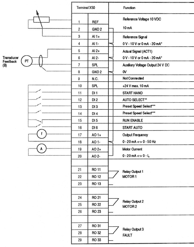
\* Selected voltage or current reference with plugs S1 and S2 on the customer interface board (beside the screw terminals 1-6 of X50).
