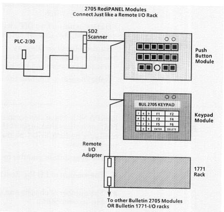
The modules are addressed through DIP switch settings in the same manner as remote I/O racks. Additional DIP switches allow you to select the following features:
