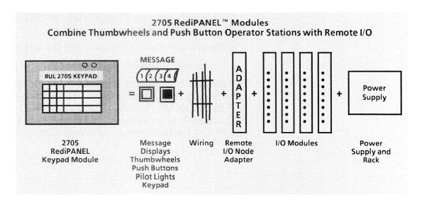
RediPANEL Modules connect to remote I/O scanners and sub-scanners just like remote I/O racks. This replaces large wire bundles with a single twin-axial cable that connects the module to the programmable controller. Up to sixteen separate modules can be located on a single cable up to 10,000 feet away from the programmable controller.
