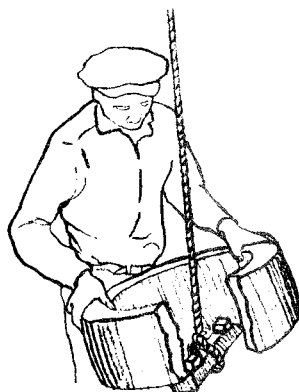
Fig. 3 Method of Handling the Bushing Current Transformer
