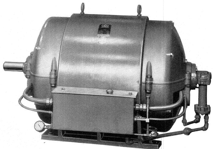
PRESSURE LUBRICATION. FIG. 27—500 hp, 3600 rpm squirrel-cage motor for oil pipe-line pumping. Lubrication is furnished by pump worm-gear to motor shaft. High-pressure side is by-passed to reservoir with pre-set orifice to control proper flow of oil. Oil rings provide oil when motor is starting up.
